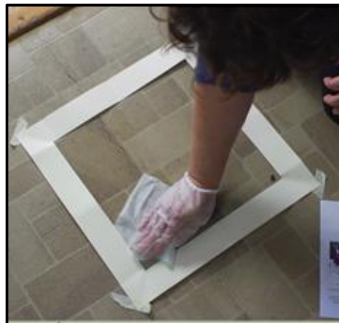
Above: Home lead dust testing involves taking samples of a square foot area of floor surfaces (shown here) and a windowsill to see if there is any lead dust present in the samples.
