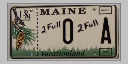
The operator who sets the dies for embossing, has a plate board as their guide for the letter and number placement and the spaces and hyphens for that plate type and design.
