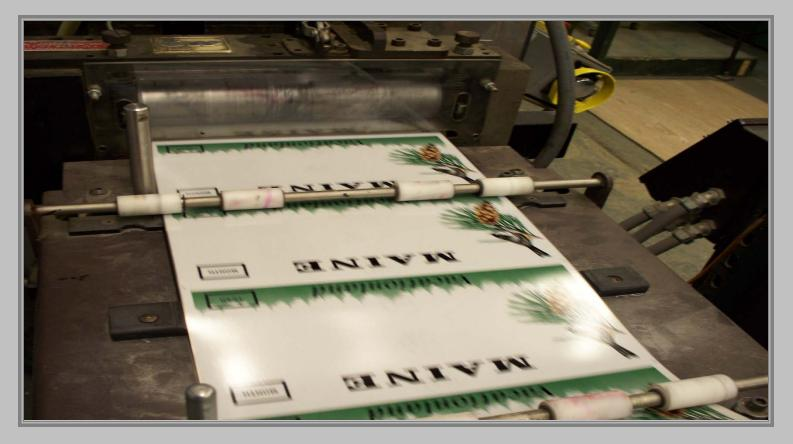
At this point, no rims, no letters or numbers are embossed, only the Scotchlite has been applied and the corners trimmed, and the holes punched.
