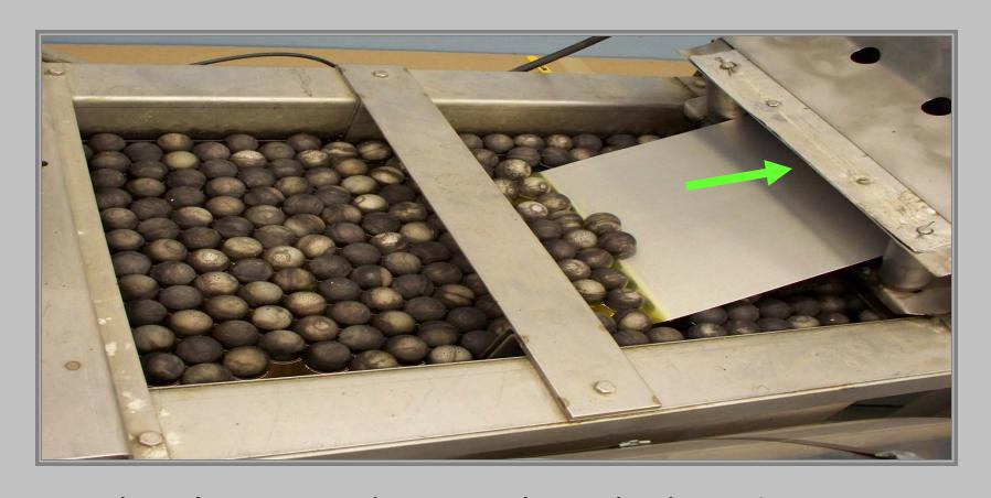
As the aluminum advances through the tub, it moves through steel rollers that press it flat and removes the dimples or any imperfections that couldn't be washed out.
