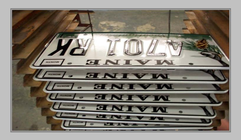
Once the rack returns from the oven, each plate is removed, checked, shrink wrapped as pairs, and strapped into 50 plate bundles or 25 pairs. The bundles are stacked on a skid pallet. (Single plates, such as trailers and motorcycles, are not shrink-wrapped, just strapped in bundles and stacked on skid pallets).
