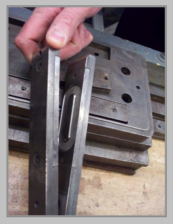
This die is the number "0". The embossing die resembles a giant clothes pin without the spring. It has a limited opening and is inserted in its place on the Embossing Press by the operator. When inserted into the Embossing Press, the blank sets inside this die, allowing the force of the machine to emboss the image into the blank.
