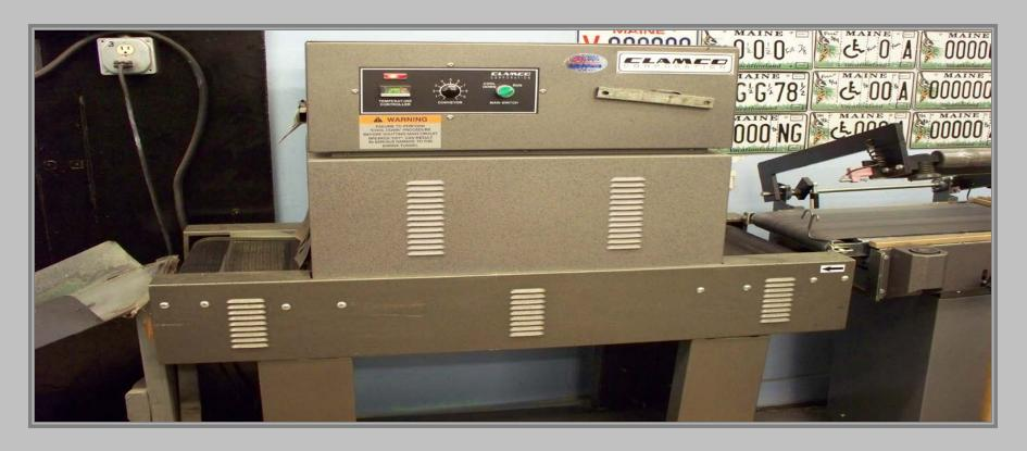
Pairs of plates must be brought to the Sealing Machine before receiving strapping. Each pair is placed on a tray and cellophane is wrapped around them. The pair proceed into the Sealer that shrink wraps the plastic to the plates as the sealed wrapped pair exits from a conveyor belt, down a shoot, and ready for bundling.
