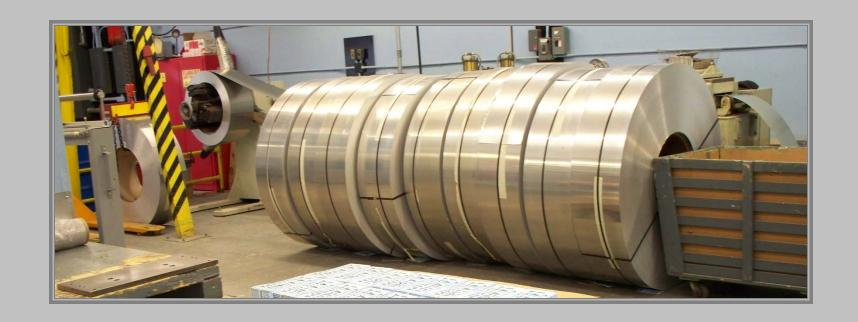
Upon entering the Plate Shop, rc'g of aluminum are in view and standing upright ready for processing. Each roll of aluminum weighs between 1,200 and 2,200 lbs.
