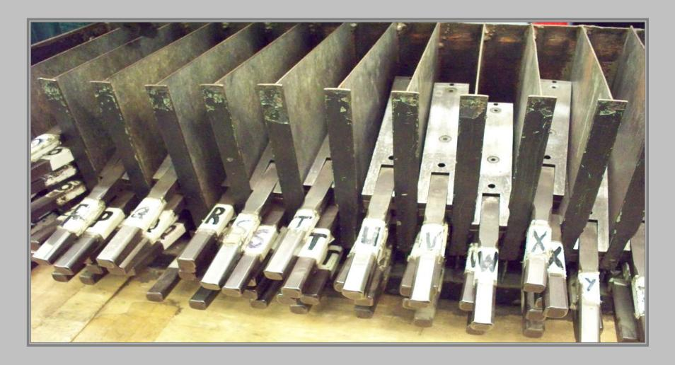
Each die is clearly marked so the operator can visibly identify the character without confusion. This process takes a great deal of concentration and coordination in conjunction with the operator feeding the blanks.
