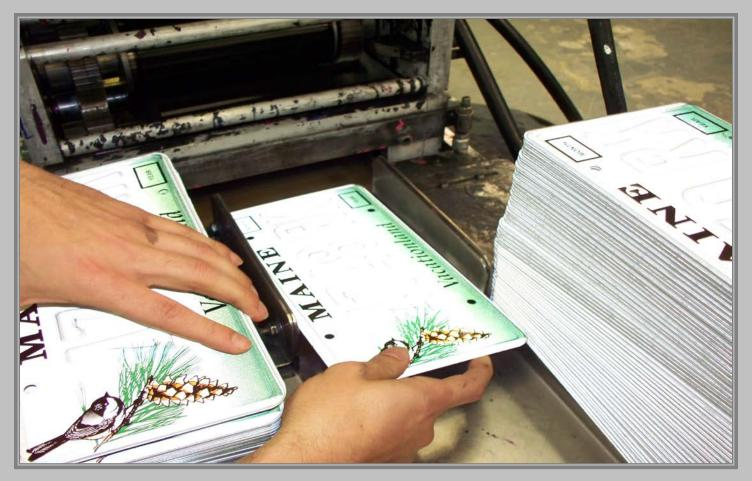
Each plate is individually placed in a slot that is belt driven through the inking machine and runs over the conveyor rollers.
