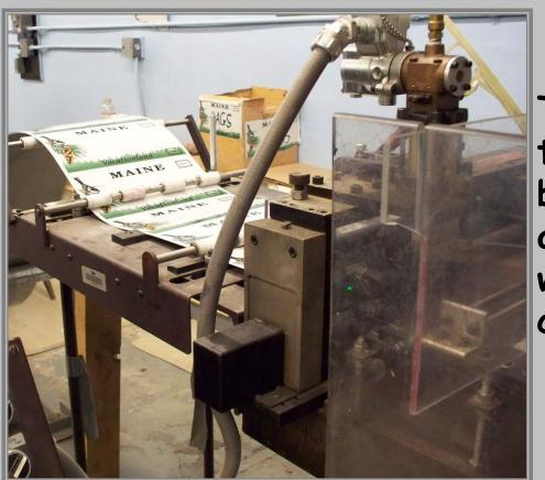
The Passenger Plate design that depicts Maine's State bird, the Chickadee, is being applied to the aluminum and will continue on its way to be cut into license plate blanks.
