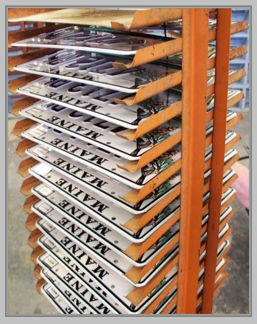
The racks are hung from a revolving monorail system that is suspended from the ceiling.
