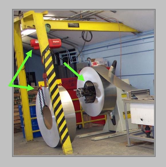
An electric hoist lifts a roll of aluminum so the roll can be placed on the Blanking Press spool. The roll is unrolled, washed, and dried in preparation for the 3M Scotchlite application, prior to the Blanking Press cutting the aluminum into plate size blanks. Thus the name, "Blanking Press".
