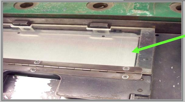
The blank will drop into a slot that positions it for the embossing, which takes place from other side of the Embossing Press.
