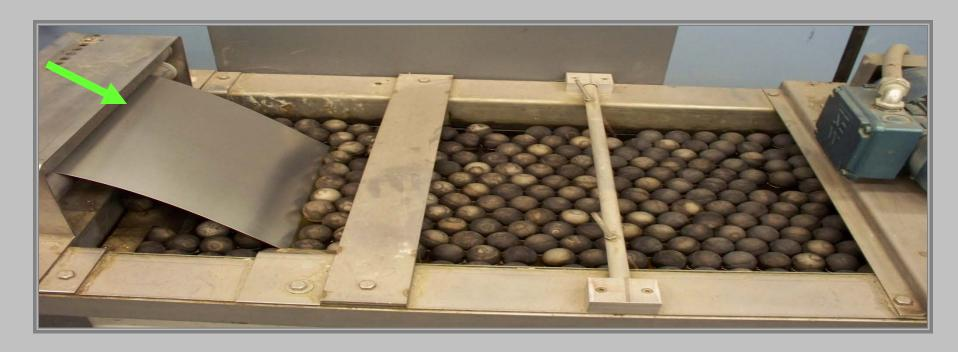
As the aluminum unrolls, it is submerged in a pre-heated (350 degree) tub of hot water. Hollow (ping-pong type) balls float on the surface of the water and assists with holding the metal under water to maintain the necessary heat and moisture to soften the aluminum. The aluminum exits through two rollers that compress the metal to remove the water as the metal is guided through the roller slot. An offset fan waves air over the top of the aluminum to assist with the drying process.
