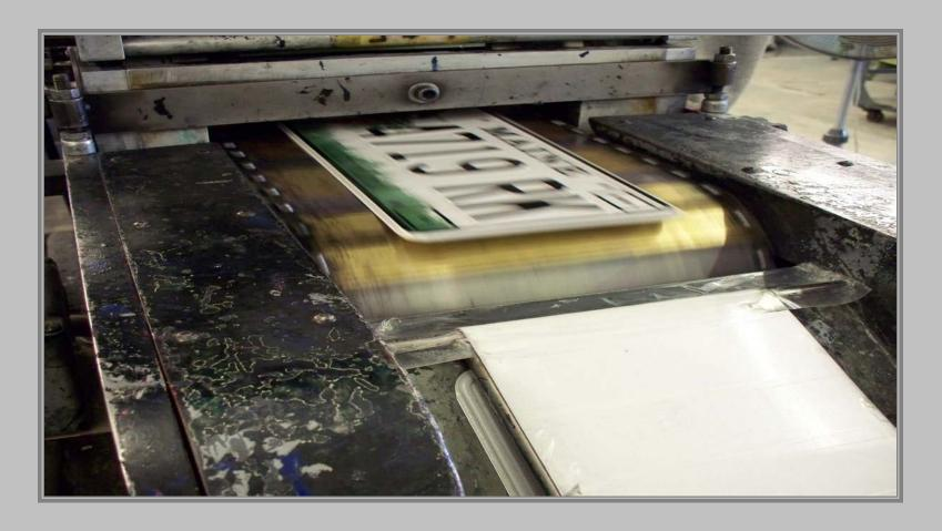
The plate passes under the ink roller and over the conveyor rollers and exits into a tray. The operator removes the plate and places it in a drying rack.
