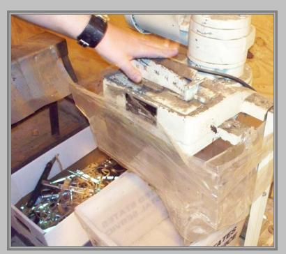
One person can shred a box of returned plates in less than 10 minutes, simply by feeding the top of the machine slot with a license plate so the machine teeth can shred them into 2, 3, or 4 pieces. The pieces drop into a bin, located under the shredding table. These shredded plates are then emptied into a dumpster for recycling along with the trimmings from the Blanking Press.
