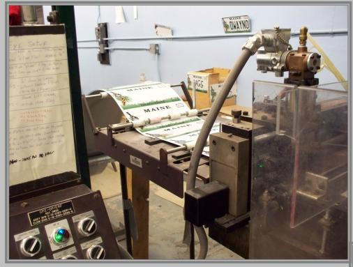
Views of the aluminum advancing to the Blanking Press to be cut, now that the 3M Scotchlite has been applied.
