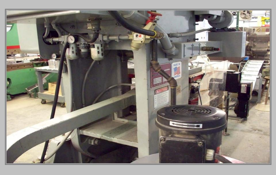
The Blanking Press, near the vacuum, as the aluminum advances to be cut into blanks.
