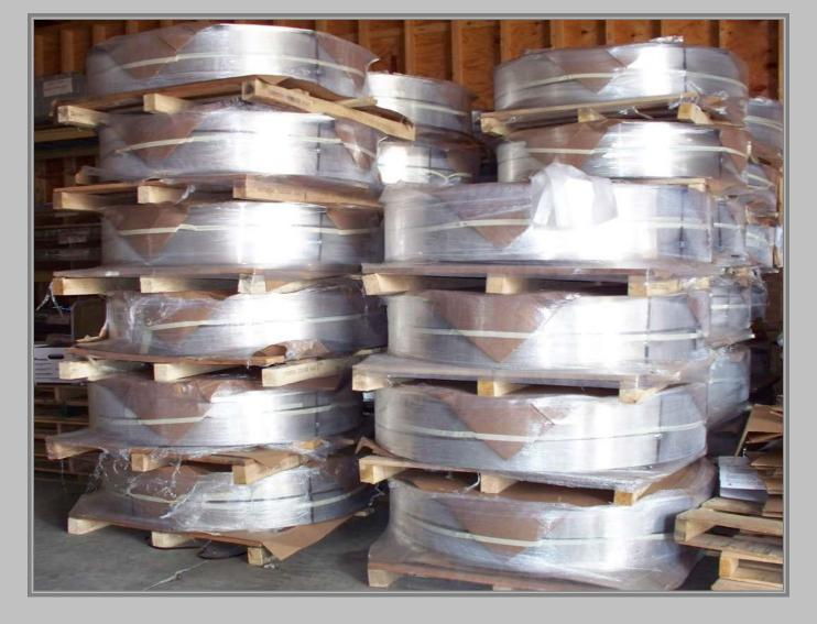
Rolls of aluminum also are stored in the Warehouse. Each roll of aluminum weighs between 1,200 and 2,200 lbs.
